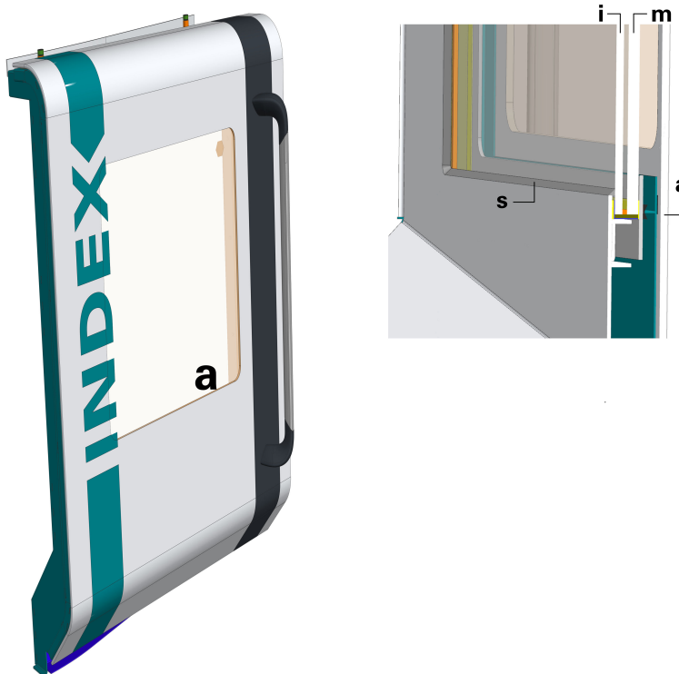
Example: MS32-6.3 window pane of work area door 1 (Fig. 1)
