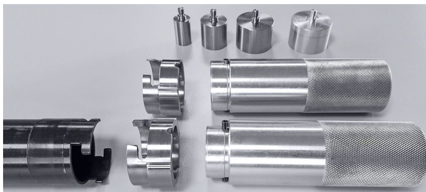
Example: Spindle liner tube and bush with mounting tool
