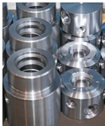
Guides (Ø 110×120 mm) and bases (Ø 75×50 mm) for cylinders used in damping technology.
