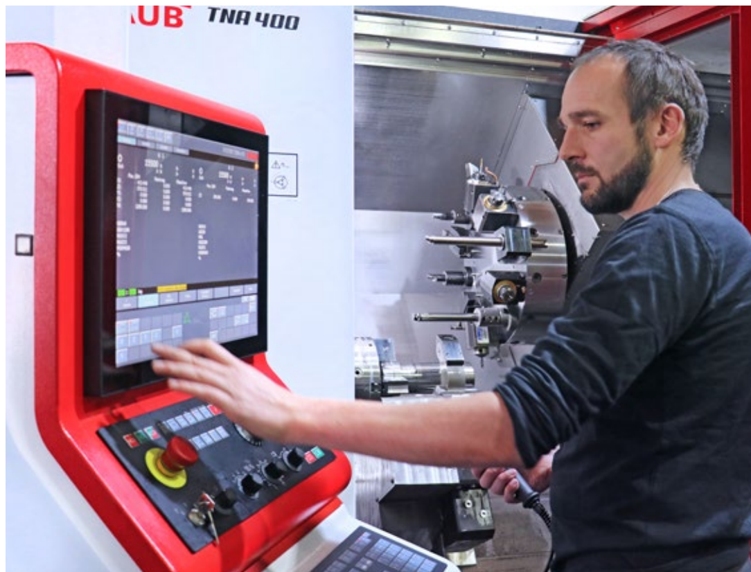
Managing Director Thomas Lieb and the new TRAUB TNA400. The universal machine is compact and easily accessible. All existing tools can be used in the typical TRAUB disk-type turret with VDI40 holders. Important components for Lieb are also the NC-controlled steady rest and the NC tailstock.
