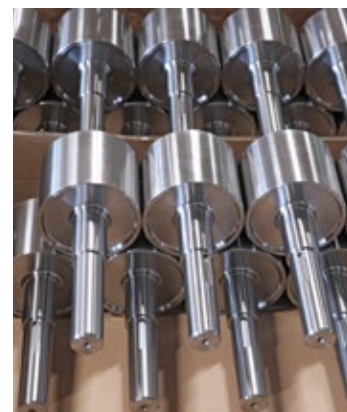
Steady rest work from solid material: The parts with a diameter of 110 mm and lengths of 125/270 mm were previously welded raw parts.
